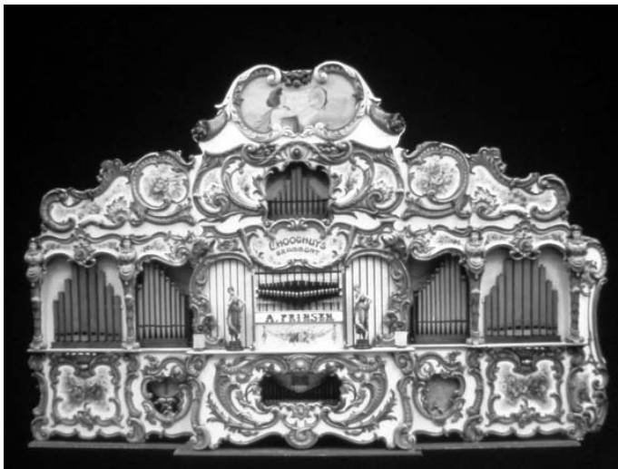
Figure 5. A Hooghuyts dance organ built in 1923. The painting is original. The organ is beautiful but not a large organ. There are not a lot of pipes—Hooghuyts have a special type of pipe—the organ can make more volume with just three ranks of pipes than other organs with five or six ranks. The mixture was specially made up with a very crisp sound. The organ is now located in Geeraardsbergen, Belgium
