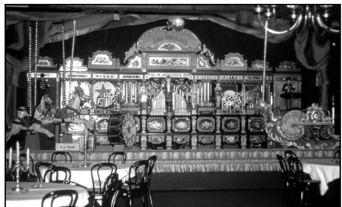
Figure 10. This was an 87-key Gavioli organ located in Tournus, France. The owner (Jean Ducloux) added extra trumpets and bass for increased volume. It doesn't exist now as one day a former worker put fire to the building the organ in which the organ was housed.
